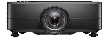
At 9800 lumens with 4K and HDR compatibility, the ZU920TST features a dust-resistant IP5X certified optical engine for 24/7 operation capabilities, offering true maintenance-free projection for up to 30,000 hours of powerful performance in Eco mode. Other features include a motorised zoom, full motorised lens shift and built-in dual 10W speakers.
